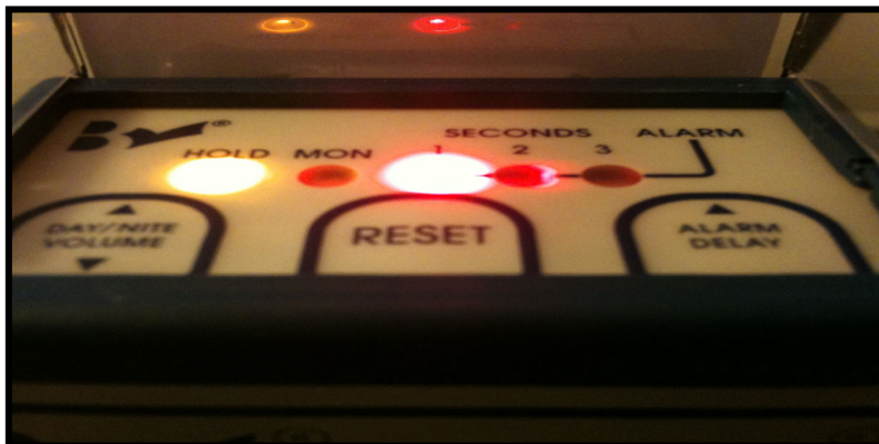
Figure B Standby Mode
