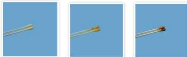
Figure 2. Examples of Unacceptable Swab Specimens for Xpert Carba-R Assay Testing:
