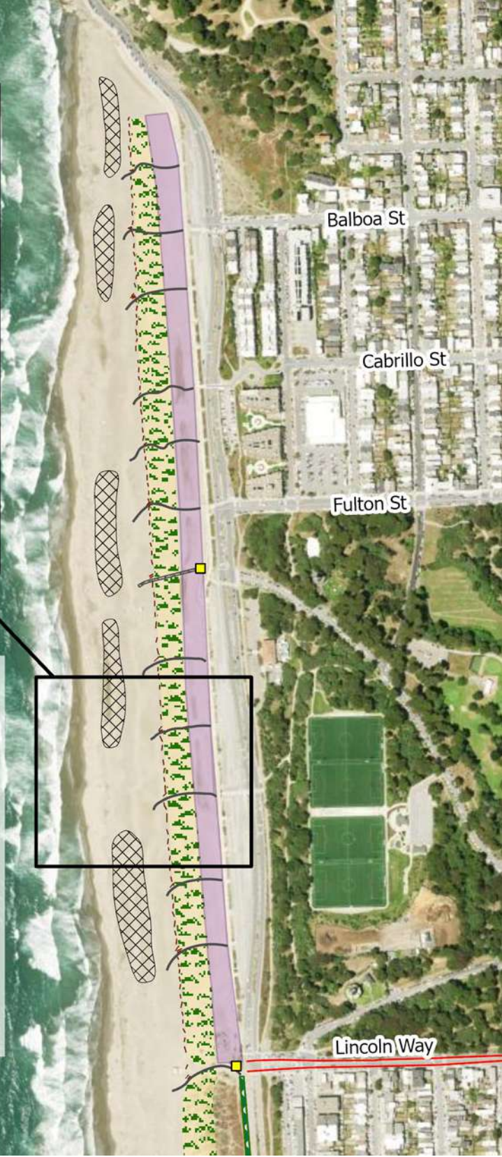
Figure 8.1. Concept design summary for Reach A. Elements can be adjusted based on management and recreational priorities; for instance, spacing of excavation troughs is flexible, and the density of pedestrian access paths can be shifted to accommodate more designated dune-crossing trails in areas with higher foot traffic or fewer trails in areas with lower foot traffic.
