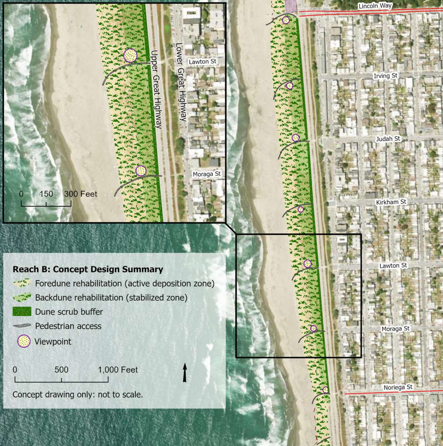
Figure 8.5. Concept design summary for Reach B. Reach B design elements focus on revitalizing the existing dunes and guiding pedestrian access to designated locations to reduce trampling.
