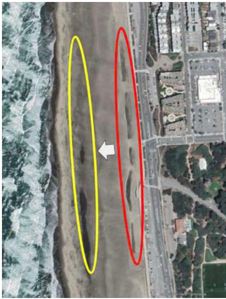
Figure 8.2 The backpass excavation is moved shoreward from the current location just seaward of the seawall (excavation pits visible in aerial photo) to the runup zone above the high tide line.
