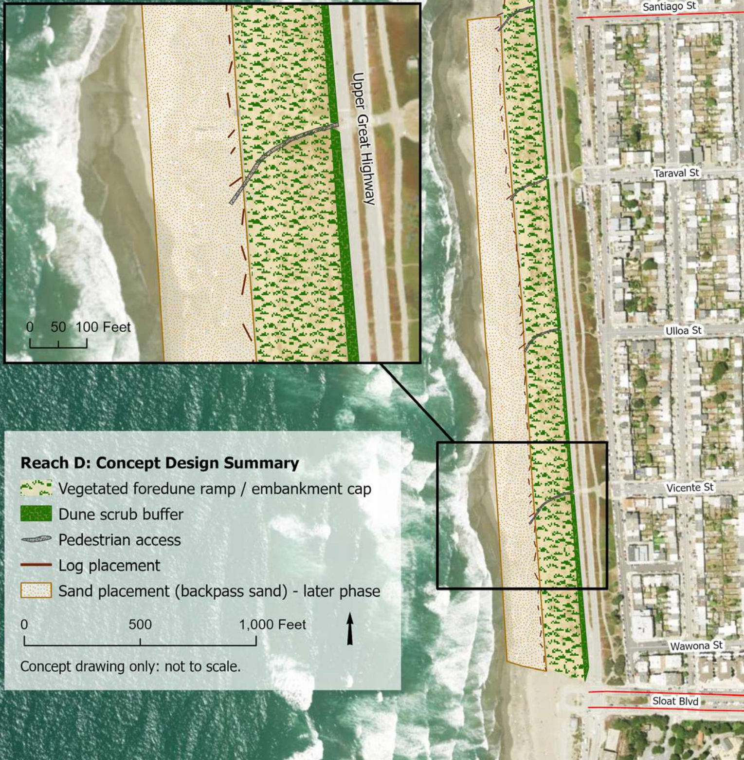
Figure 8.7. Concept design summary for Reach D. Once vegetation is established, backshore sand placement can help nourish the dunes.
