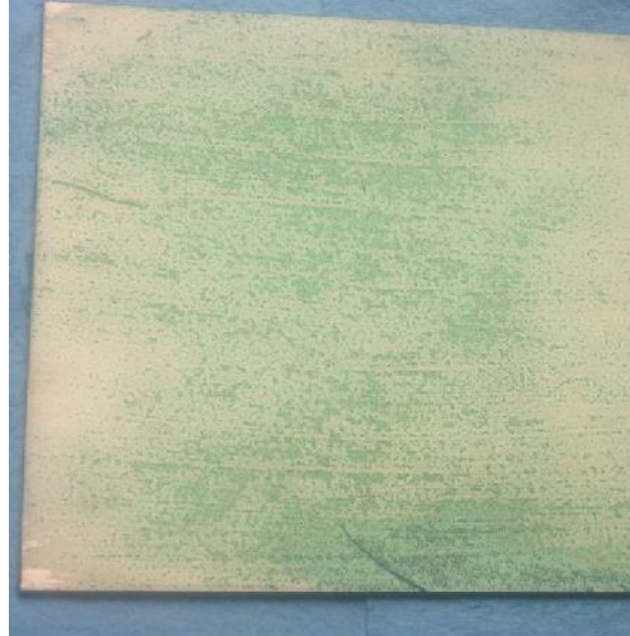
Photo 1 - Dura-Grip initial application w/o lacquer
