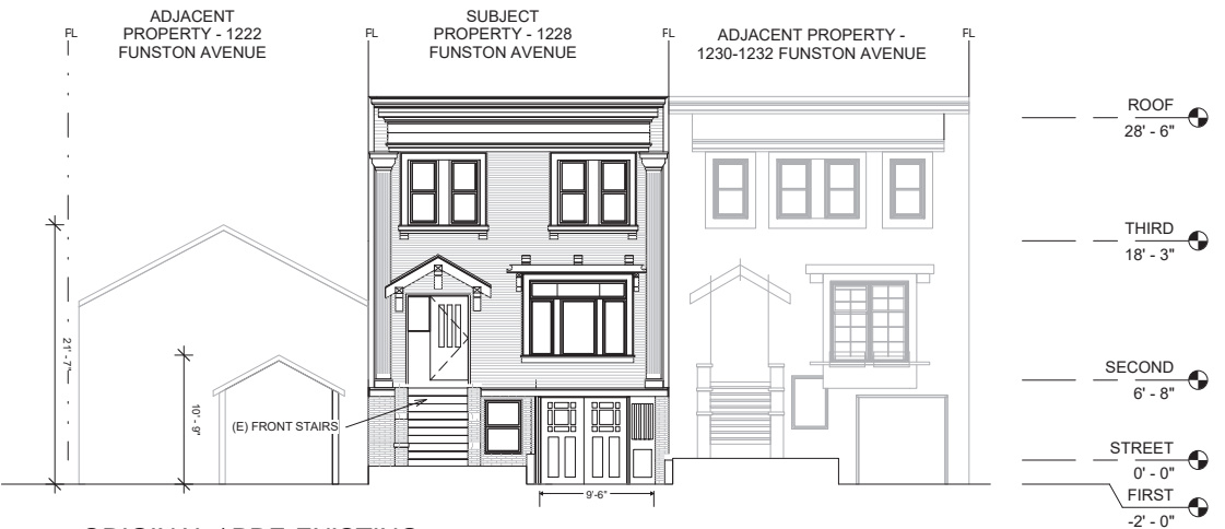
ORIGINAL / PRE-EXISTING SCALE : 1/8" = 1'-0" WEST ELEVATION
