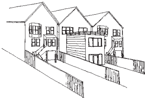
This addition has been scaled back to two stories and is set in from the side property lines to minimize its impact.
