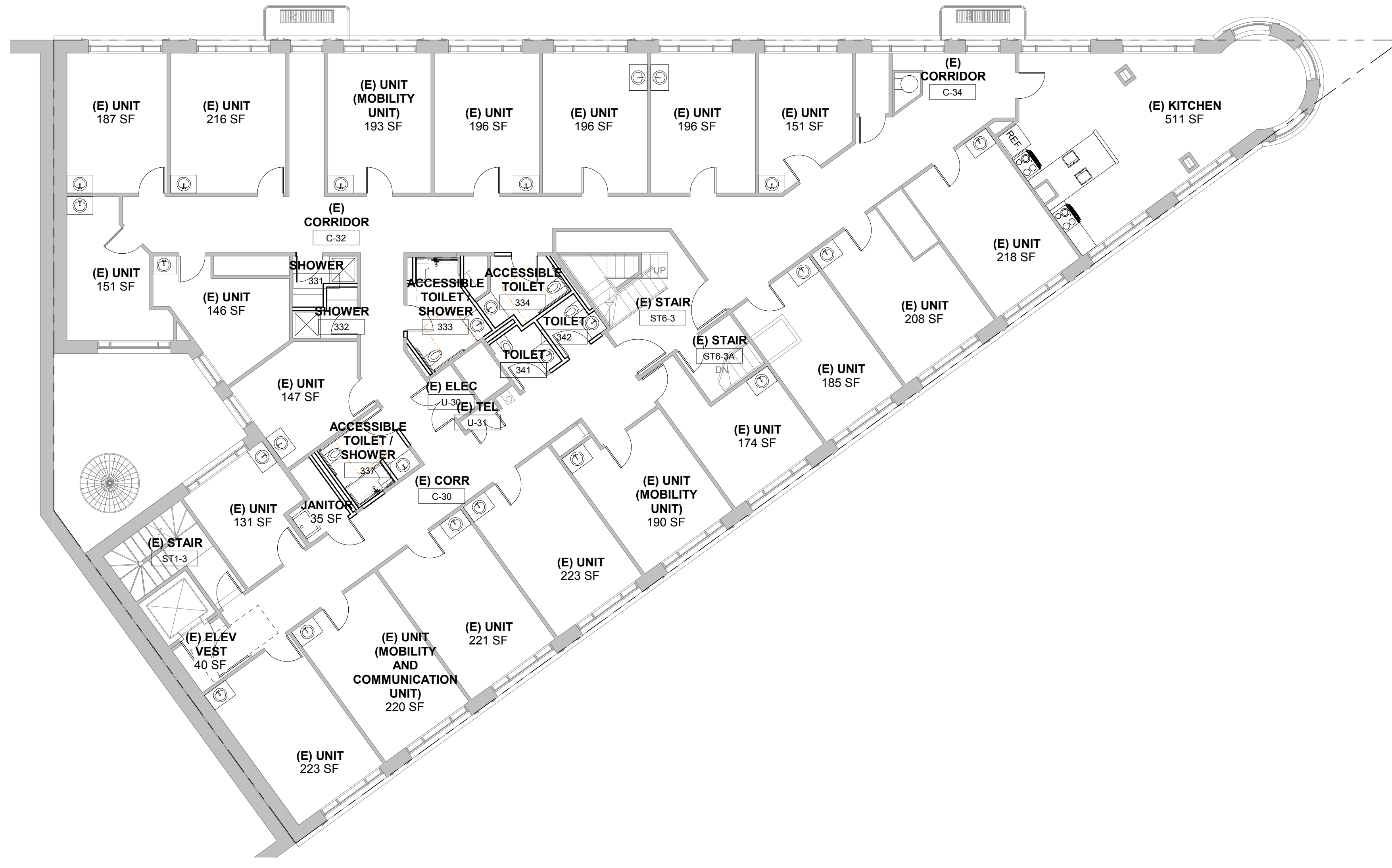
LEVEL 03 FLOOR FIRE SAFETY AND EXIT PLAN 2 1/8" = 1'-0"
