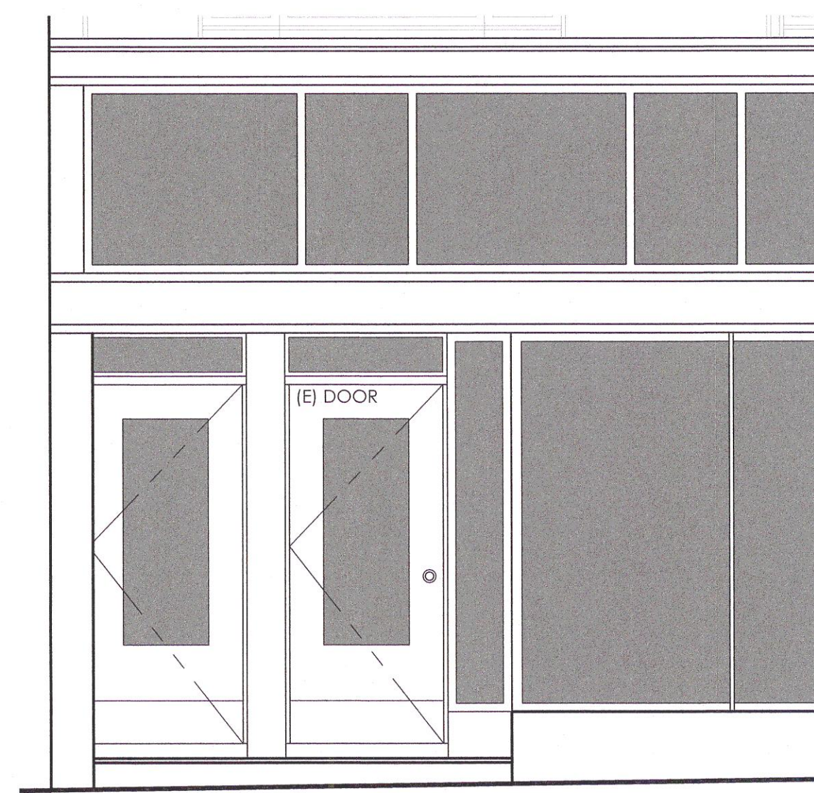
3 ENLARGED PARTIAL EXISTING/DEMO ELEVATION 3/8" = 1'-0"
