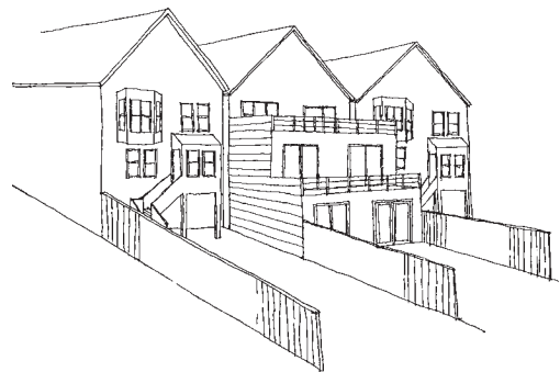
This addition extends the full width of the lot but is set back at the second floor so the building steps down to the rear yard.
