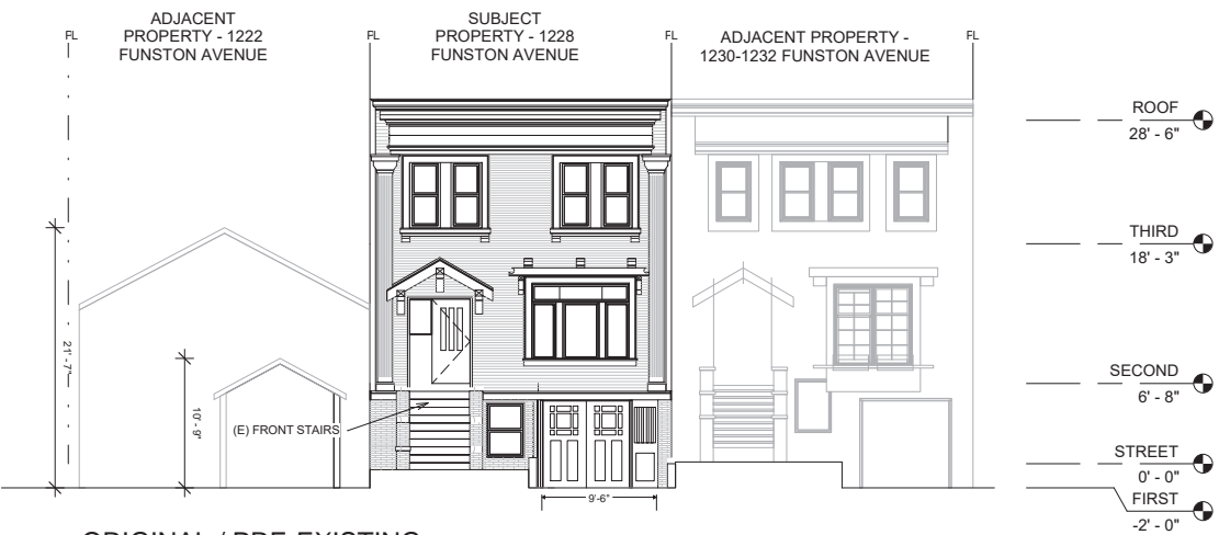
ORIGINAL / PRE-EXISTING WEST ELEVATION SCALE : 1/8" = 1'-0"
