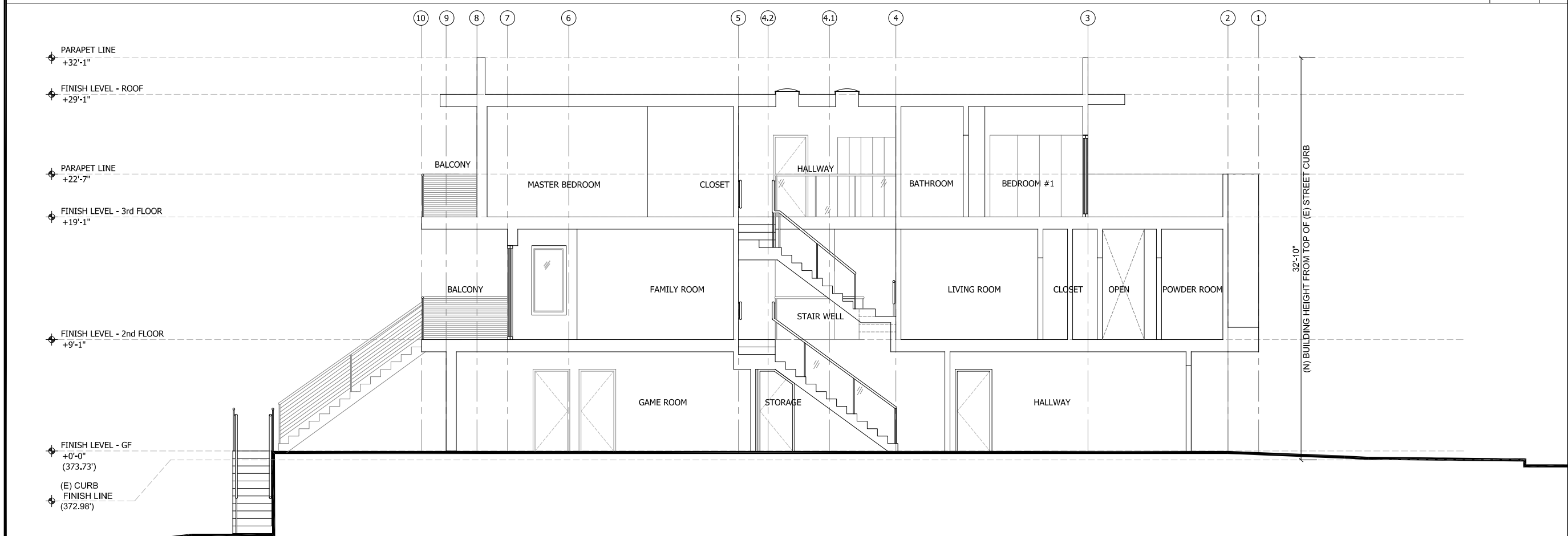
SOUTH RESIDENCE - PROPOSED EW SECTION LOOKING NORTH
