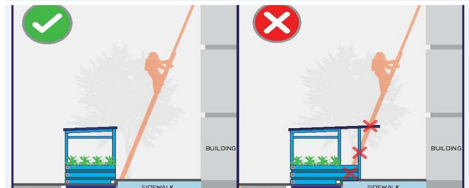
Clearance for Firefighting Ladders
