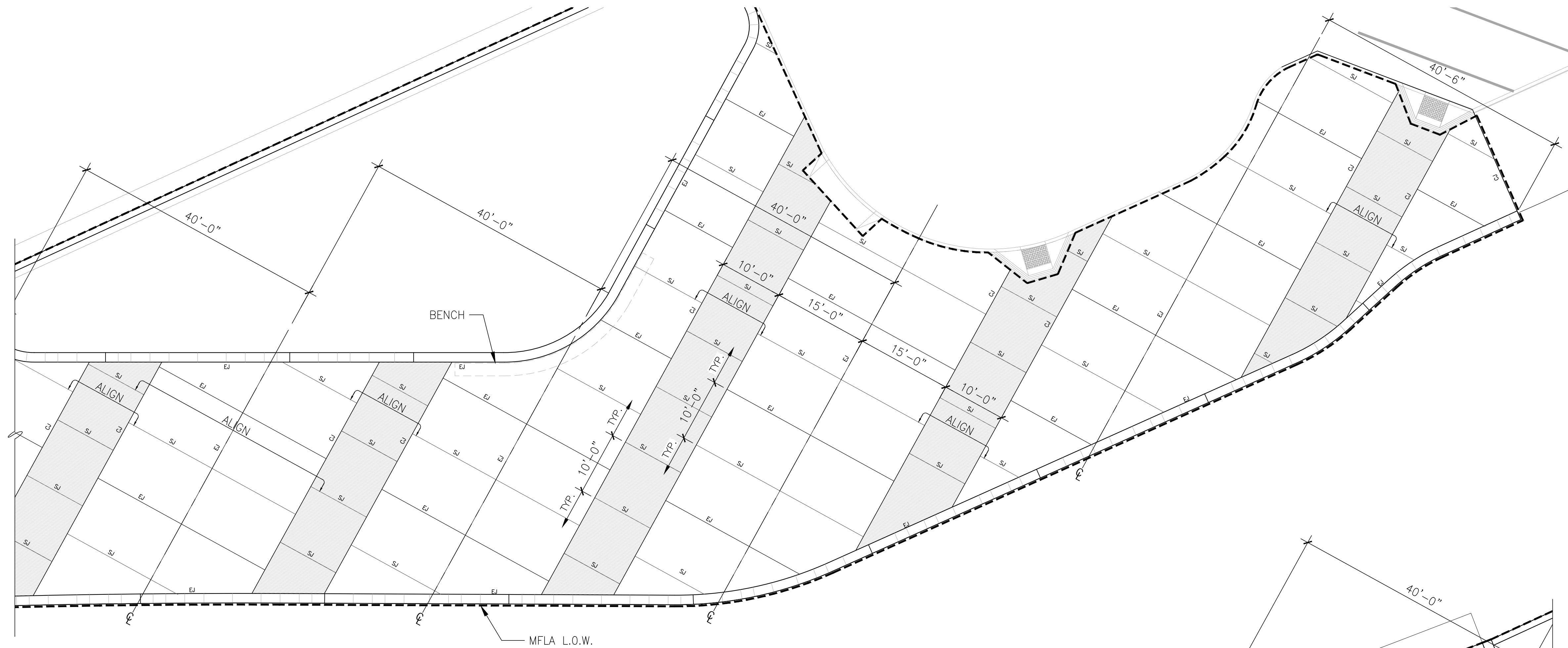
1 JOINTING PLAN SKYLINE DROP-OFF SOUTH 1" = 10'-0"
