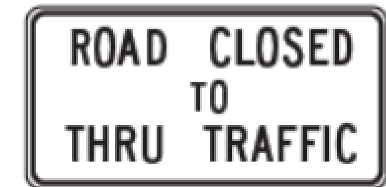
"Road Closed to Through Traffic" (R11-4) Sign
